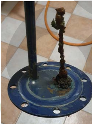
One of the consequences of electrochemical corrosion is rapid anode loss, which is why the first anode replacement is justified at 12 months, so in case of significant loss, the problem can be identified in time without damaging the storage body (18 months after that).
